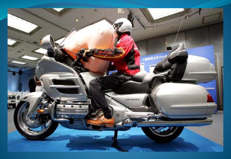
What is the airbag inflated with? Nitrogen gas. The reaction that makes an airbag inflate is:  $2NaN_3(s) \rightarrow 2Na(s) + 3N_2(g)$ Nitrogen gas fills the airbag, but sodium is also produced – if sodium reacts with water (in a person's mouth or eyes = very bad and caustic). So designers added other chemicals to react with Na and make it safe.
