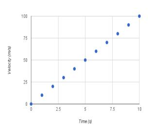
The slope is 10 m/s per second.  $\frac{rise}{run}$
