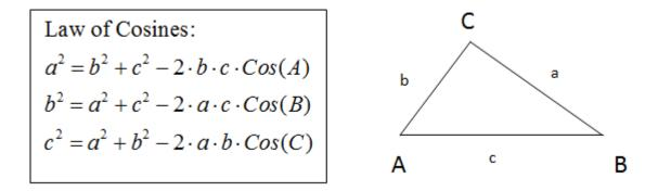
EG: A surveyor needs to find the length of a swampy area near Fish Lake. She sets her transit at point A. She measures the distance to one end of the samp as 468 m (point B) and the distance to the other side of the swamp as 692 m (point C). The angle between the two points ( $\angle A$ ) is 78°. Determine the length of the swampy area to the nearest meter.
