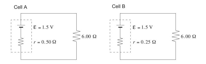
With supporting calculations, state which cell delivers the greater power to the  $6.00 \ \Omega$  resistor. (7 marks)
