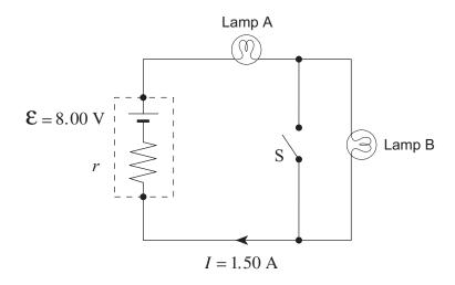
a) If a current of 1.50 A flows in the circuit, what is the internal resistance r of the battery? (4 marks)
