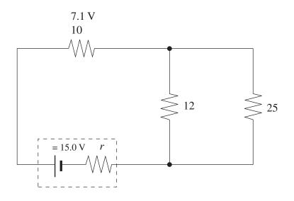
a) What is the power dissipated by the 25 resistor? (4 marks)
