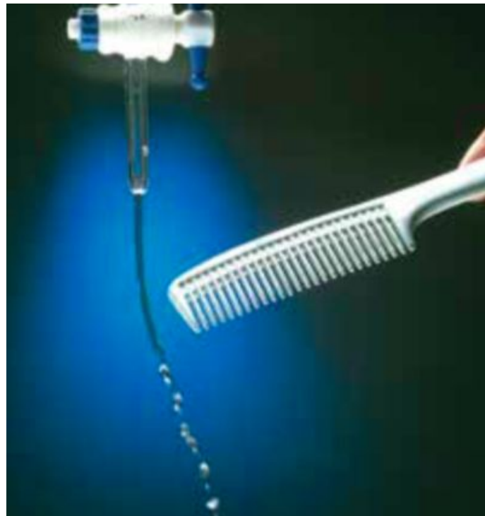
Figure 3.11: The comb is charged, and the water is neutral.
