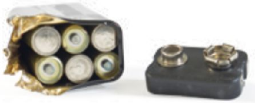
Figure 3.14: The battery shown here is made up of six individual electrochemical cells.
