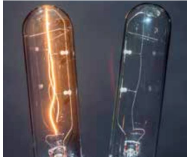
Figure 3.18: A light bulb is a load because it converts electrical energy into heat and light energy.
