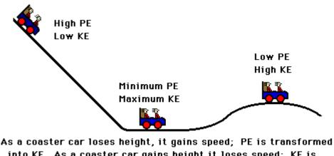
into KE. As a coaster car gains height it loses speed; KE is transformed into PE. The sum of the KE and PE is a constant.
