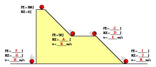
Answer: The only force doing work is gravity. Since it is an internal or conservative force, the total mechanical energy is conserved. Thus, the 100 J of original mechanical energy is present at each position. So the KE for A is **50 J**.
