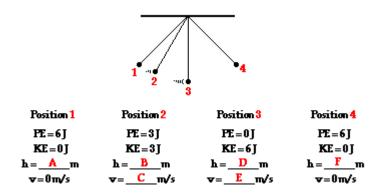
As the 2.0-kg pendulum bob in the above diagram swings to and fro, its height and speed change. Use energy equations and the above data to determine the blanks in the above diagram.
